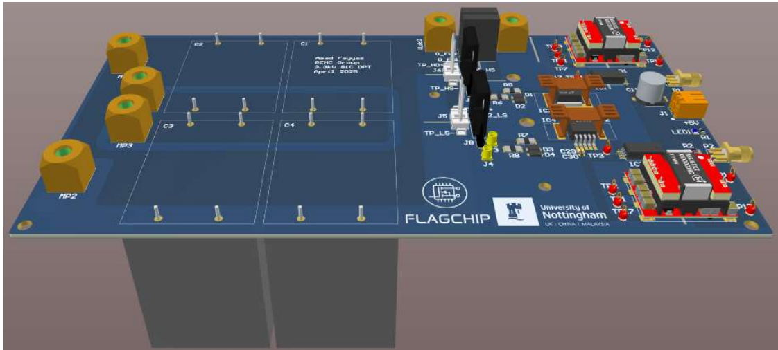
Figure 3: Dedicated PCB for dynamic switching tests for FLAGCHIP project
