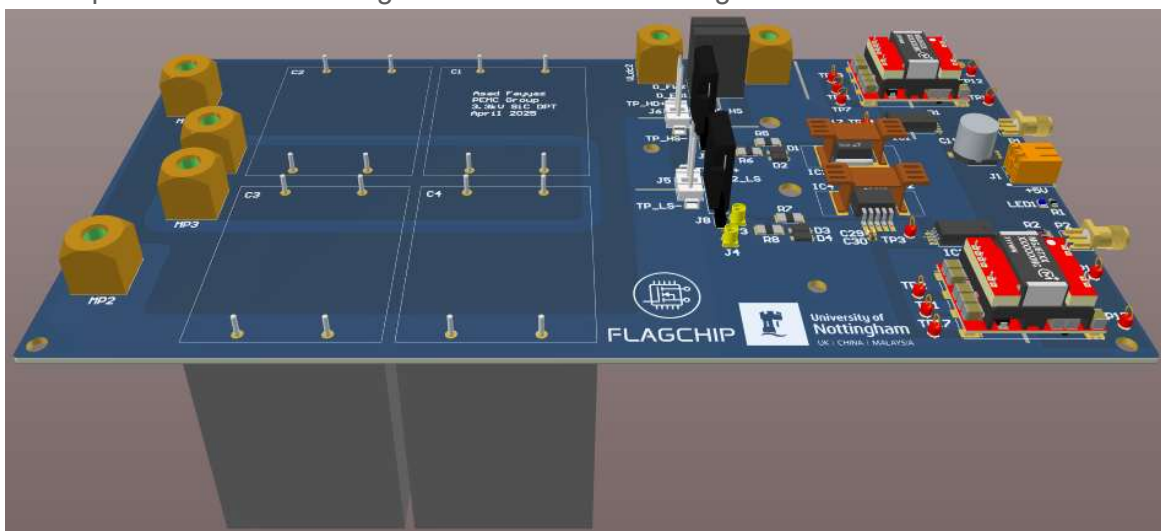
Figure 1 : Dedicated PCB for dynamic switching tests for FLAGCHIP project
